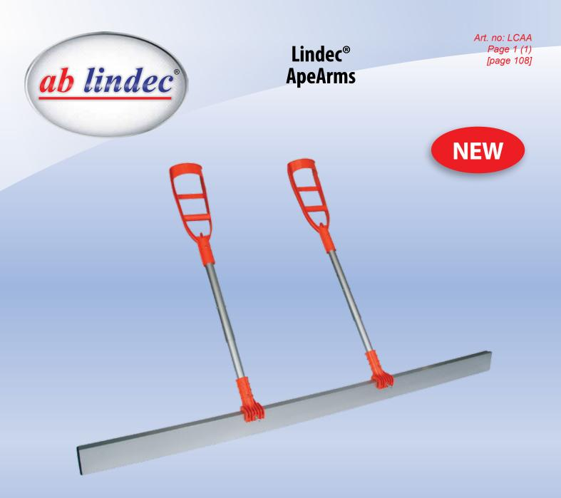
Ergonomic screed handles, which enables you to stand «upright» and don't have to bend your back or sit on your knee's, while screeding concrete, sand, or soil when placing stone or making other soil works. The gab in the opening is 38 mm.
