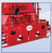
Forklift pockets for safer lifting.
