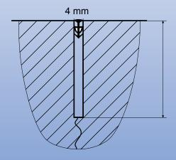
**Cutting depth** 1/4 - 1/3 of slab thickness
